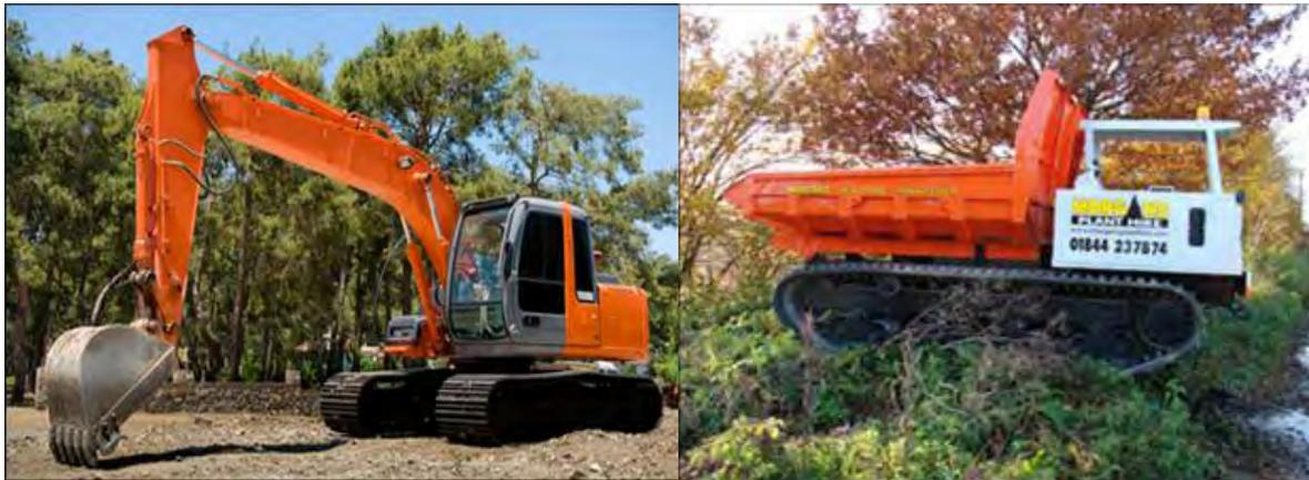
**Figure 2.21 Typical Excavator and dumper used in OHL foundation installation**
