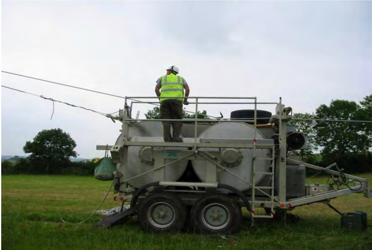
**Figure 2.33 Puller – Tensioner machine**
