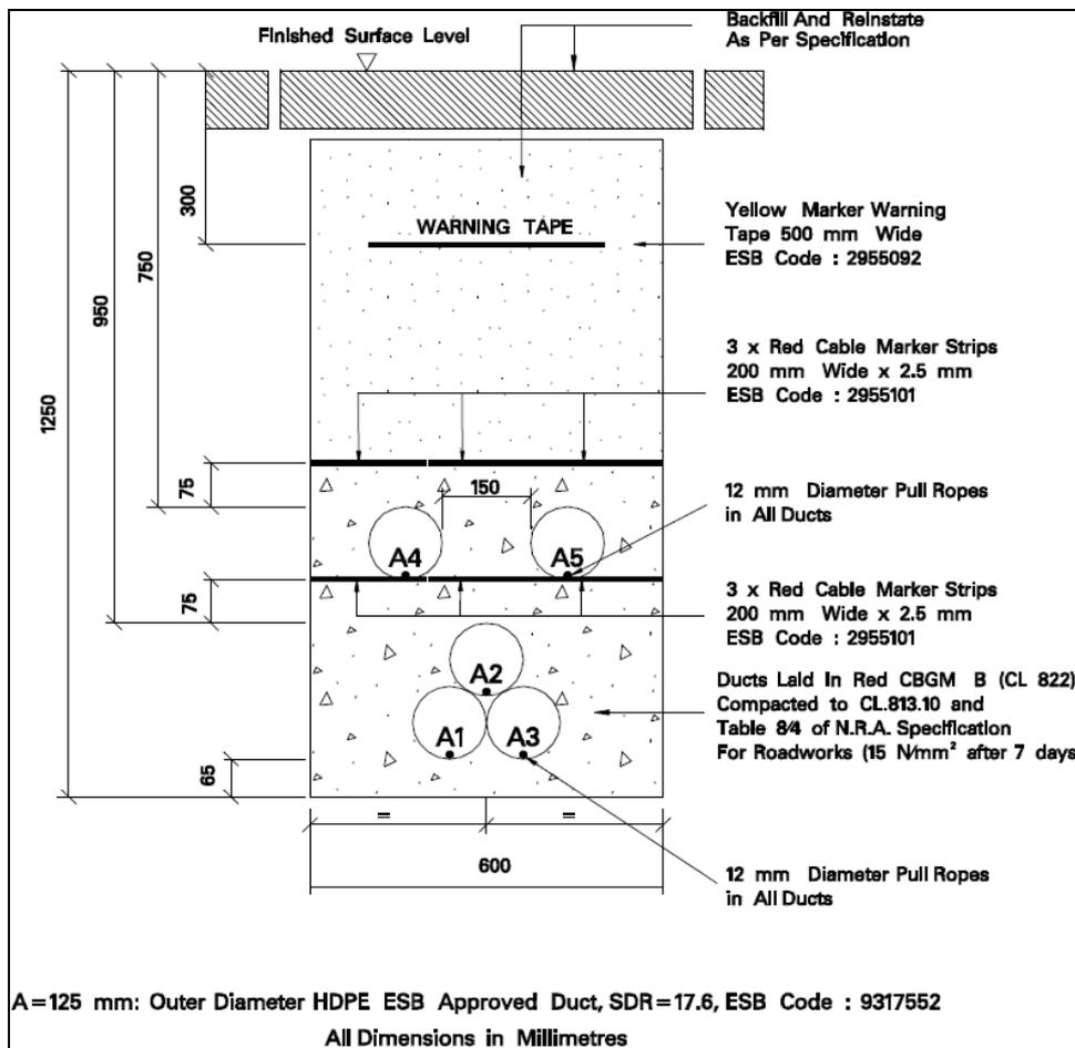
Figure 2.36 Trench Cross Section – 110 kV Single Circuit Trefoil 5 way duct formation
